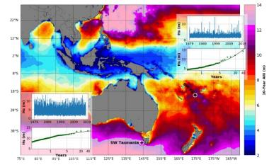
10-year average return interval (ARI) significant wave height (Hs), calculated from a generalized pareto (GPD) fit of all hourly data for years 1979 –2018 tiles in the map region. Two example locations, south-west (SW) Tasmania and south-west (SW) Fiji archipelago illustrate the full hourly timeseries (upper plots) and empirical and fitted ARI values (green circles and black lines, respectively, in lower plots), both sites are plotted on the same scale.
