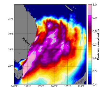
Extent of waves during East Coast Low in June 2016 normalised by 1-in-50 year wave height. Extract data, calculate statistics, combine grids and make plots in ~20min.
