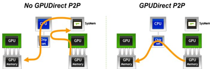
Figure 1: P2P GPUDirect Configurations (Image credit: VMWare)
